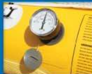
Wibit Manometer (pressure gauge)
